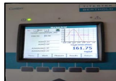
C. Concentration of DNA obtained through Nano-drop
